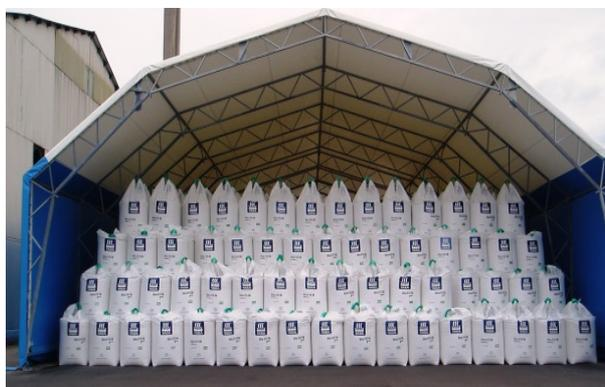
PORTABULK® FIBCs typically consist of a load-bearing outer - manufactured from woven Polypropylene (PP) - and an inner barrier component – made from Polyethylene (PE) film.
