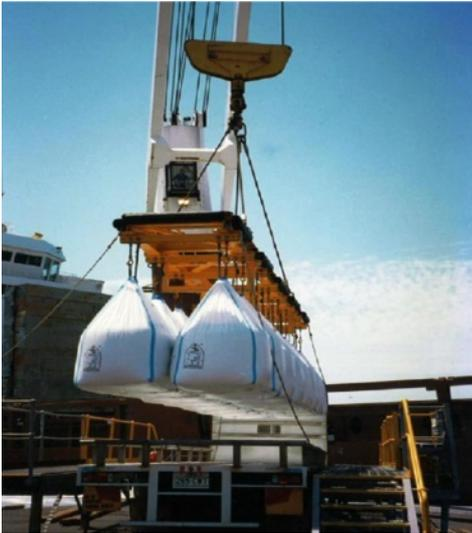
Portabulk® FIBCs currently available can be designed with 1-loop, 2-loops or 4-loops lift; typical sizes range from 500 - 1 500 kg SWL; they can be utilised and are certified for either non-Dangerous Goods or Dangerous Goods purposes; they can be certified for “single-trip” or “multi-trip” applications; they can be used in conjunction with palletised and reeled filling systems and they can handle most bulk commodities, from fluidised powders to heavyweight particles.
