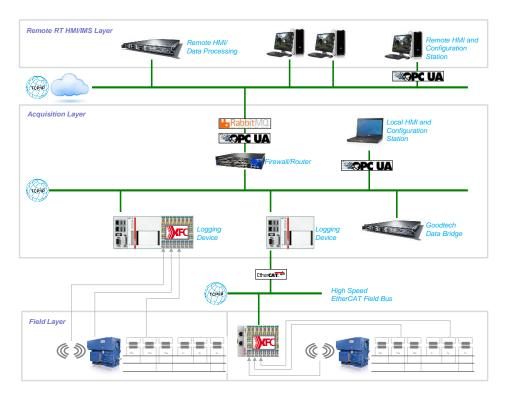
The figure shows the Goodtech System for high speed data acquisition and data processing. The system can acquire data at a speed up to 1 MHz using oversampling technology.
